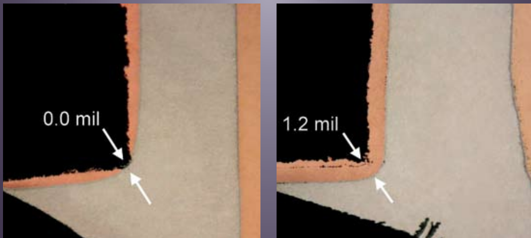
Connector after conventional SAC 305 rework showing copper dissolution (left), and minimal copper dissolution (right) using new SAC 305 rework method.
